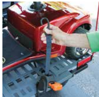
Self-tensioning retractable securement belts.
