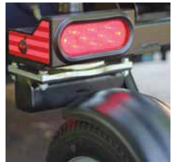
Running/brake lights and turn signals.
