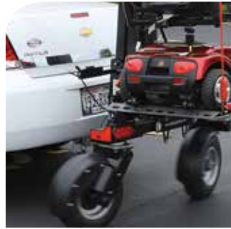
Swivel wheels, independent suspension.
